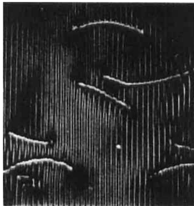
FIGURE 1 The aspect of the discontinuities at a voltage near the Williams domains threshold U_w .
